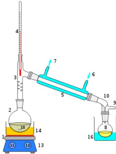
► The essence of distillation is to heat a given liquid until it became vapour and then condensing the vapours the material is converted to liquid again. Since there is no chemical alteration in the material structure, only phase transition, **the distillation is a physical process.**
