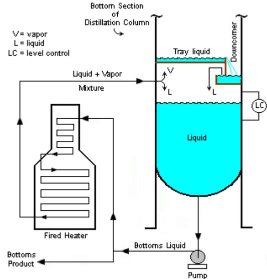
Thermosyphon reboiler (vertical)
