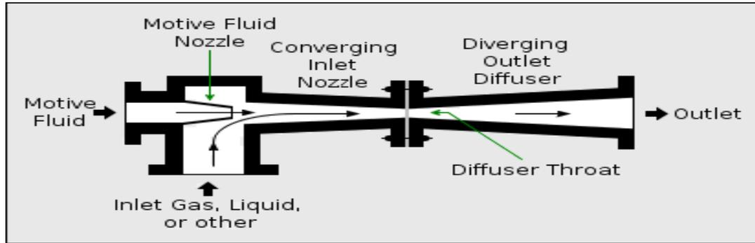
▶ The theory is that the speed (with that the moving energy) of the steam entering the converging nozzle will increase due to converging. The increased moving energy is balanced by decreased pressure. The pressure in the space around the nozzle will decrease so gas will be sucked into the nozzle from the surrounding space. In the diverging diffuser the moving energy will decrease and the pressure will increase again.
